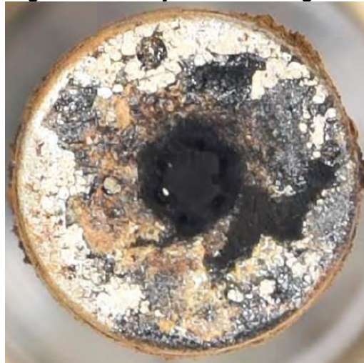
Figure 1: Fuel Injector Face Image at EOT
