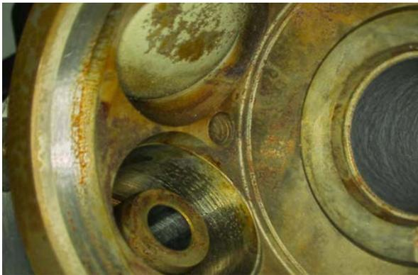
**Figure 7: Metal housing of common rail pump with iron formate deposits<sup>16</sup>**
