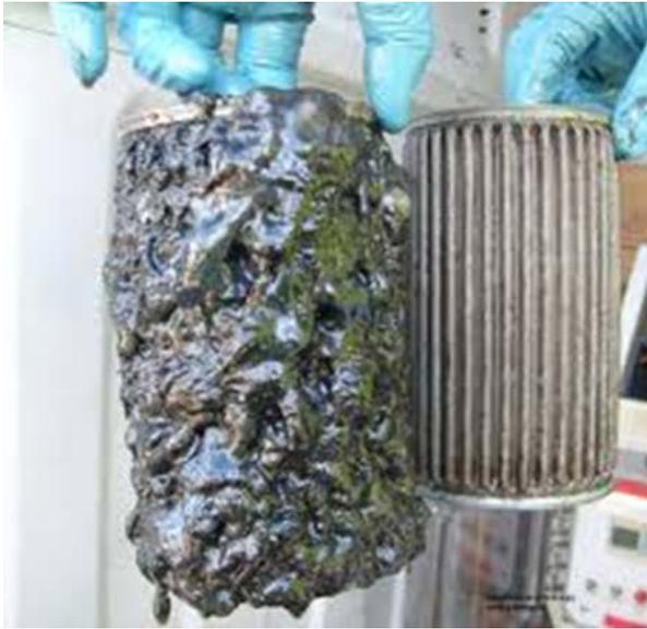
**Figure 3: Microbial plugged dispenser filter compared to a filter with no microbial contamination<sup>7</sup>**
