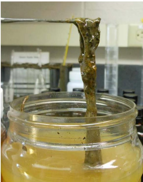
**Figure 4: Fuel "rag" layer from diesel bulk storage tank bottom sample<sup>8</sup>**
